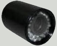
The **WPC-2.5ZIR** camera is an infrared illuminated, waterproof, day/night, zoom camera. with a 10x optical zoom. With sufficient external lighting the camera operates in the color mode, providing maximum detail. When using the internal infrared illumination, the camera operates in the more sensitive BW mode.
