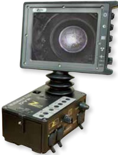
The Zistos WalkAbout® is a body-worn, 5.6" LCD Display with a built-in DVR, and on-screen indicators for battery life and LED intensity. It's battery-powered and weatherproof.
