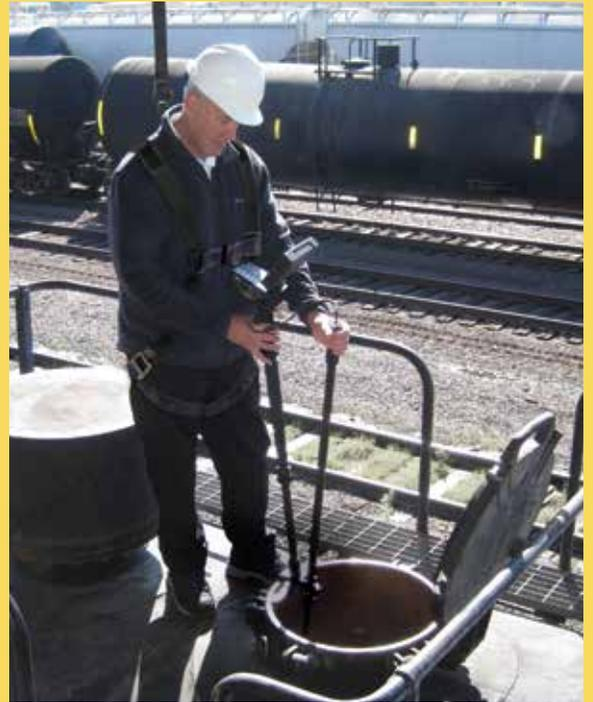
*Rail tanker inspection with Zistos Tanker Inspection System Part # IAD-TIPZ-A6*
