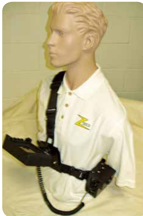
WalkAbout LCD mounted on chest plate with the WalkAbout base on waist strap. Walkabout base may be worn on belt is desired.
