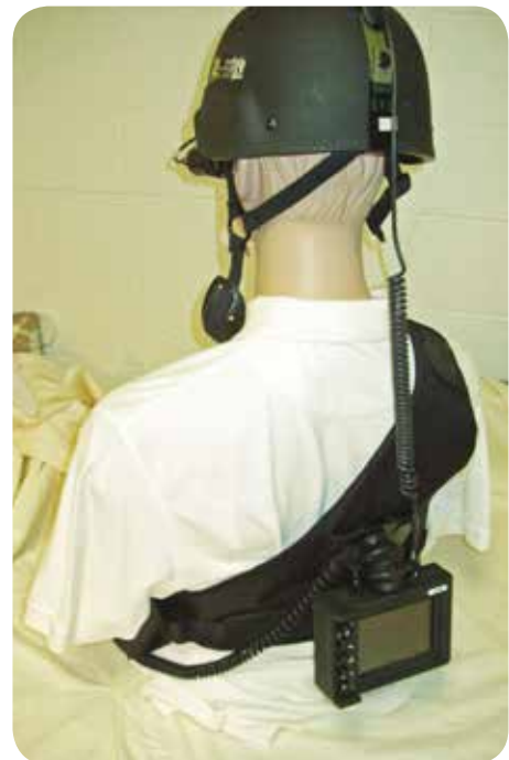
WalkAbout LCD mounted on the rear. WalkAbout base can be mounted on chest plate to balance weight making it more comfortable to wear.
